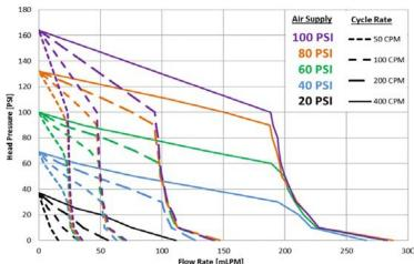
\* 300 mL/min at wide open flow path. The Flow Chart measurements shown are using a back pressure regulator to simulate a pressurized system; results may vary.
