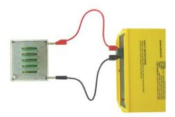
By knocking on the plate, the iron filings show the pattern fields around a current-carrying coil.
