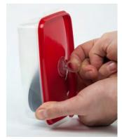
Hold the container tight and pull on the suction cup. A negative pressure is generated, which is indicated by the pointer deflection to the left.
