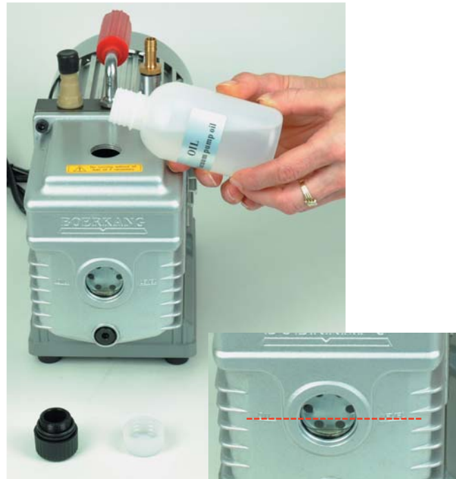
2. Fill in the oil (added) carefully and slowly until the optimal oil-level is reached (the optimal oil level is marked left and right next to the bull's eye)
