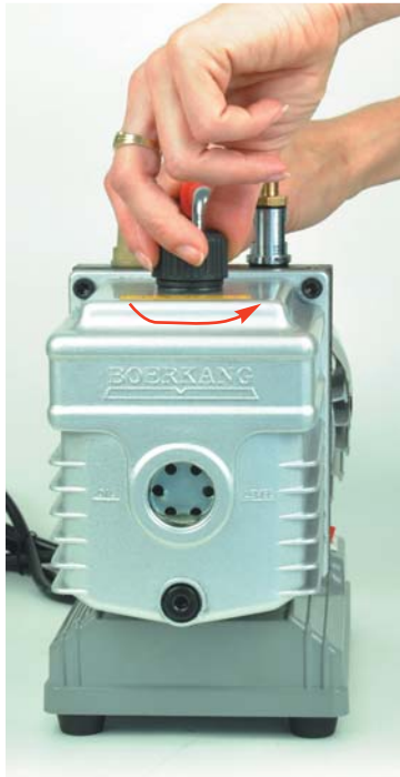
1. Open the screw cap
